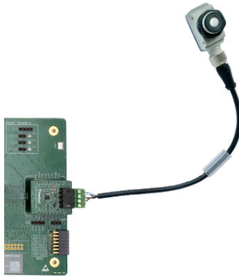
Figure 16: Distance sensor connected to the Daughterboard 0-10V
