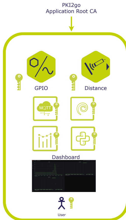
Figure 7: PKI2go provides certificates for each application component and users
