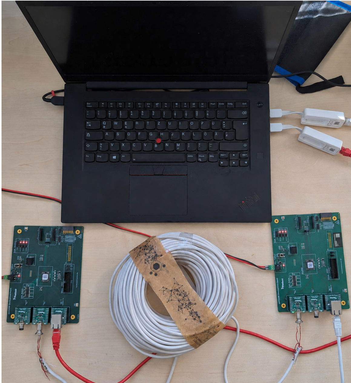
Figure 3: Physical setup of the two periCORE Development Boards and the DUT.
